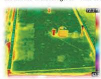
moisture trapped in the roof system and leaks in the roofing and building envelopes. Experience and understanding of roofing materials and installation procedures are used in conjunction with
